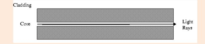
Single Mode is used for a single source of light (one colour) operation.
