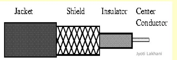
The distance between the **Outer** conductor (shield) and inner conductor plus the type of material used for insulating the inner conductor determine the cable properties or impedance.
