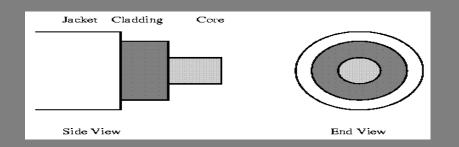
The typical optical fiber consists of a very narrow strand of glass called the **Core**.
