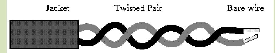
The degree of reduction in noise interference is determined specifically by the number of turns per foot.
