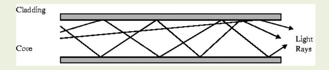
The core refracts the light and guides the light along its path.
